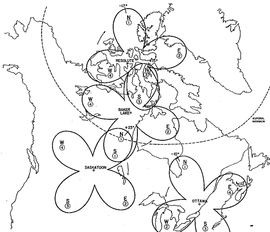
Figure 1. The locations of the auroral radars in the Canadian IGY network. The cloverleaf patterns represent the simultaneous, successive antenna beam positions of the synchronized network. The beam patterns are scaled to represent the approximate geographical coverage, out to 1140 km range.
